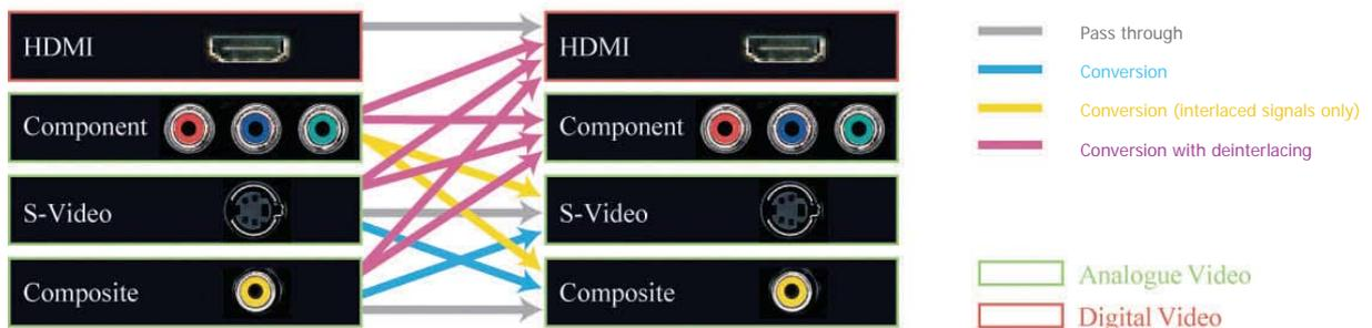
This diagram shows the conversion possibilities of a typical HDMI AV Amplifier that uses both an HDMI repeater and has HDMI upconversion facilities with a deinterlacer. Market examples would be the Yamaha RXV1600 or Yamaha RXV1700. An AV amplifier that did not perform any video conversion would only perform the signal transfers drawn in grey above.
