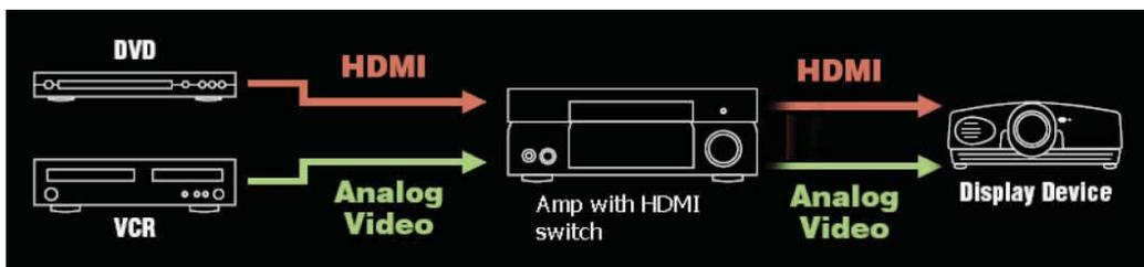
HDMI video is not processed in any way so extra input and output cables are required as no video conversion is possible
