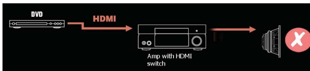
HDMI audio can not be processed in the amp so can not be heard at the speakers - additional cabling is required
